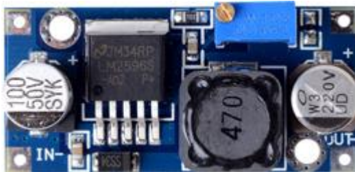
Figure 15 Shows LM2596 buck converter
