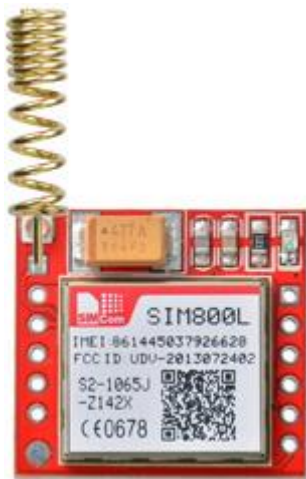
Figure 12 Shows SIM800L Helical antennae
