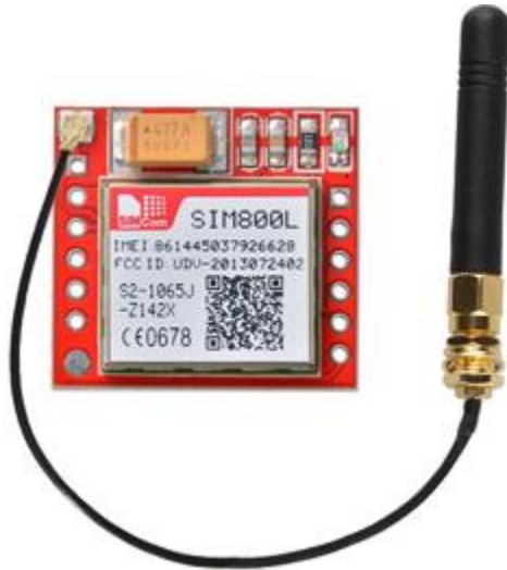
Figure 13 Shows SIM800L 3dBi GSM antenna along with a U. FL to SMA adapter
