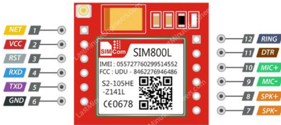
Figure 14 Shows SIM800 modem pin out
