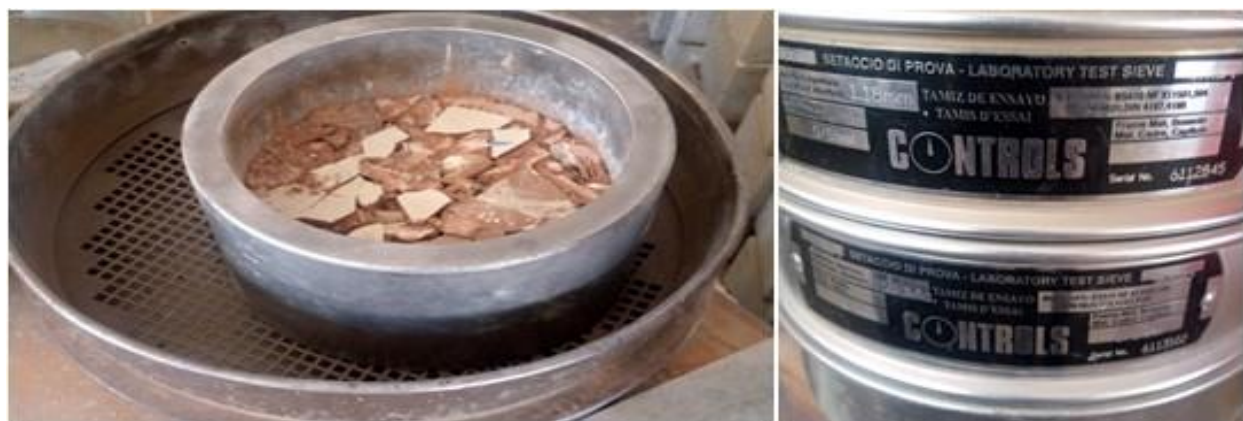
Figure 3.4: Setaccio Di-Prova laboratory test sieve at Central laboratory Ministry of works and transport-Uganda
