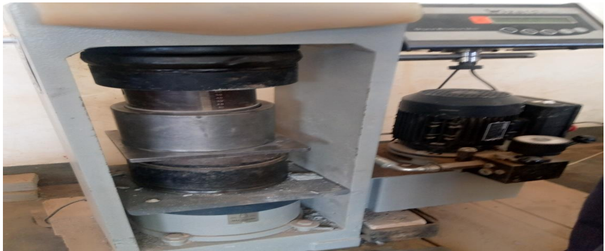
Figure 3.3: Semi-automatic uniaxial and triaxial test system at Central laboratory ministry of works and transport- Uganda
