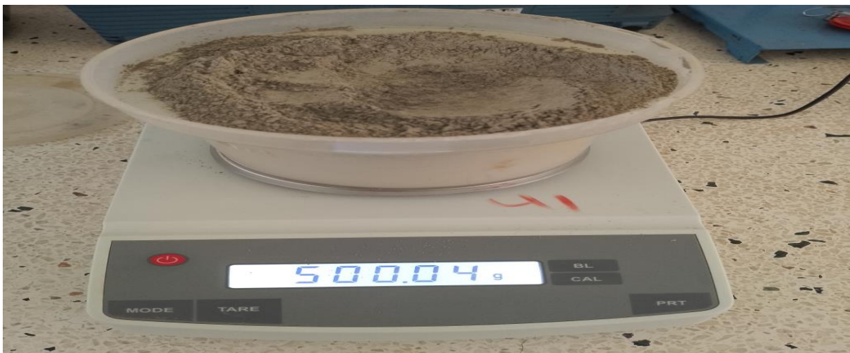
Figure 3.6: Measurement of mass of the cement samples using digital balance.
