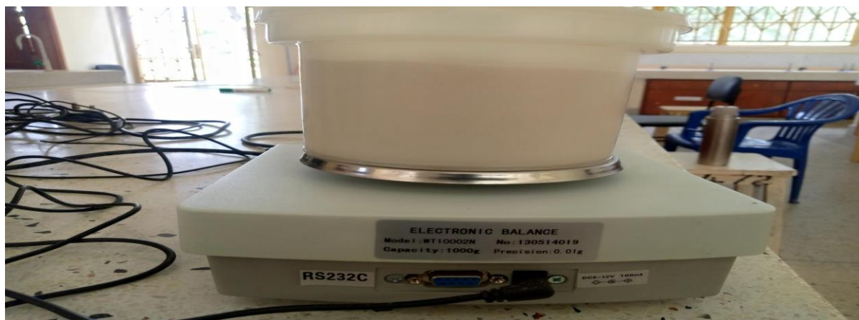
Figure 3.5: Measurement of mass of the floor tile samples using digital balance.
