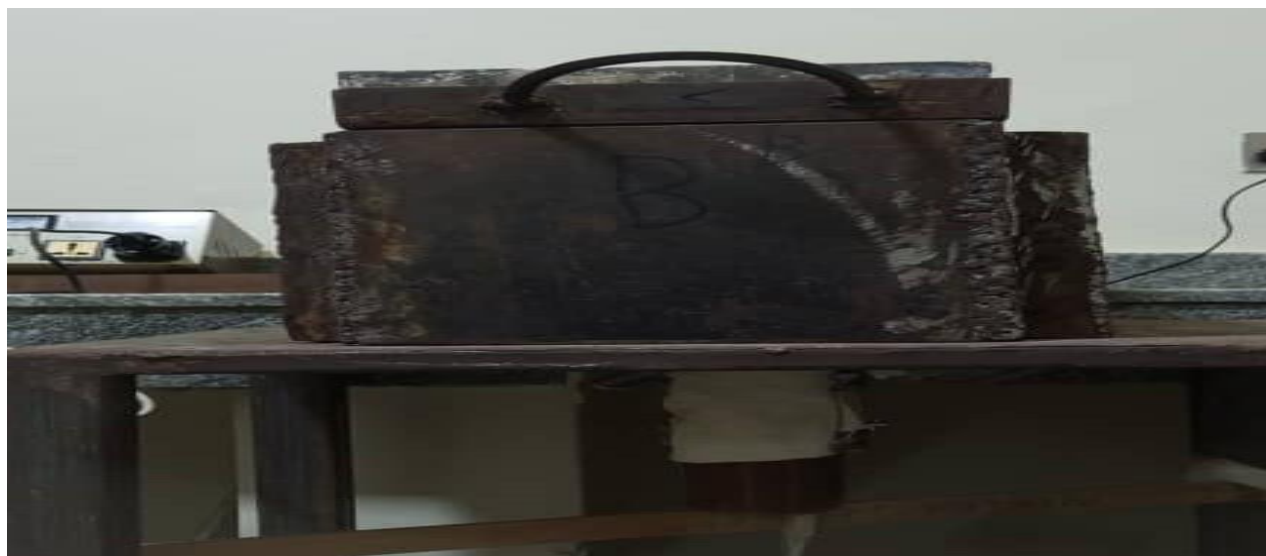
Figure3.8: A setup of lead blocks in an iron frame around the detector.
