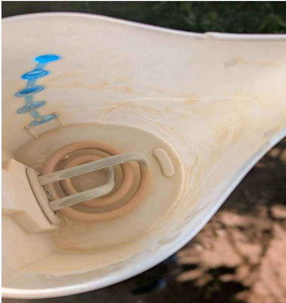
Figure 3.3:Scaling formed on the heating coil due to hard water
