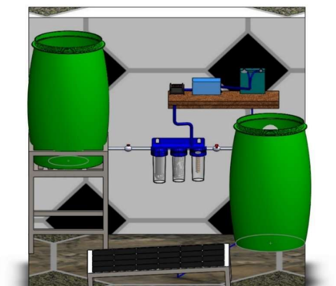
Figure 3.5: Design concept of the water softening system
