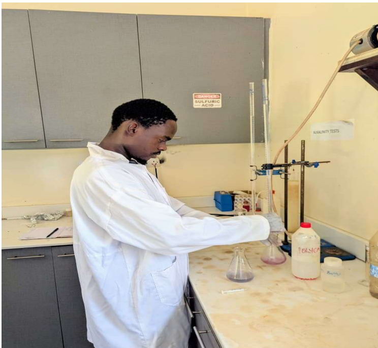
Figure 3.4:Carrying out EDTA test to determine hardness of the raw borehole water
