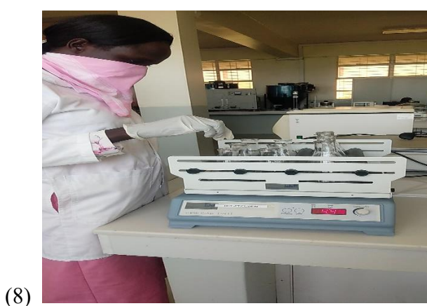
Figure C.7&8: Preparing Batch experiments and Assembling samples on orbital shaker
