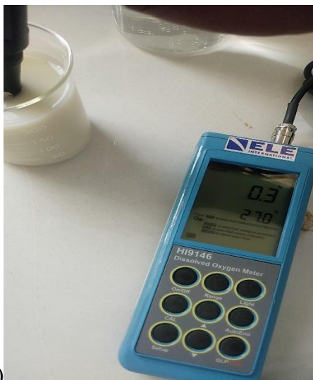
Figure B.0.2&2: HI9146 Dissolved Oxygen meter and JEN WAY 6705 Vis Spectrophotometer
