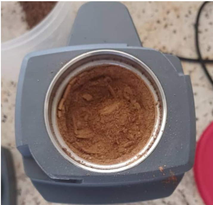
Figure 10: Powdered Dried Pineapple Peelings and Hydrochar
