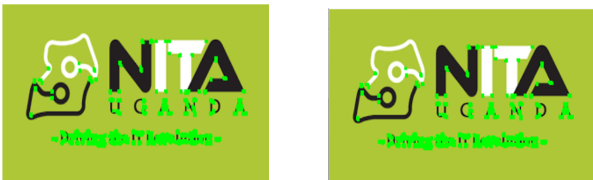
Figure 4.15: Harris Corner Detection on Cover Image (Left) and Stego Image (Right) — Corner density and distribution are visually identical
