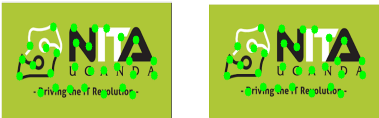
Figure 4.11: Shi-Tomasi Corner Detection on Cover Image (Left) and Stego Image (Right) — Corner locations and counts are visually indistinguishable
