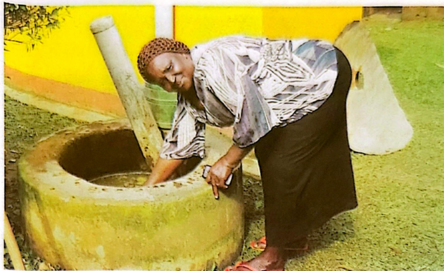
Odwar (L) mixing the cowdung with other additives such as poultry droppings, vegetable manure before pouring in the digester where biogas is generated. (R) she lights her gas cooker with biogas. PHOTO BY ALICE ADIKIN
