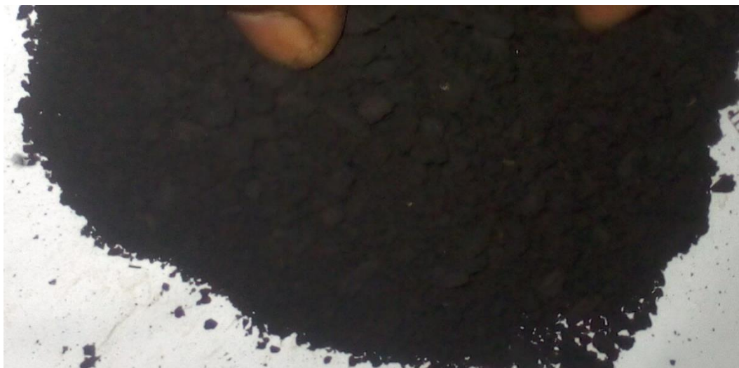
Figure 3. 5Dried Ethylenediamine-Functionalized Carbon Dots
