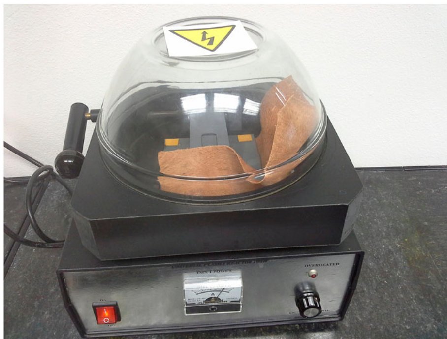
Figure 1. Universal plasma reactor with bark cloth fabrics.
