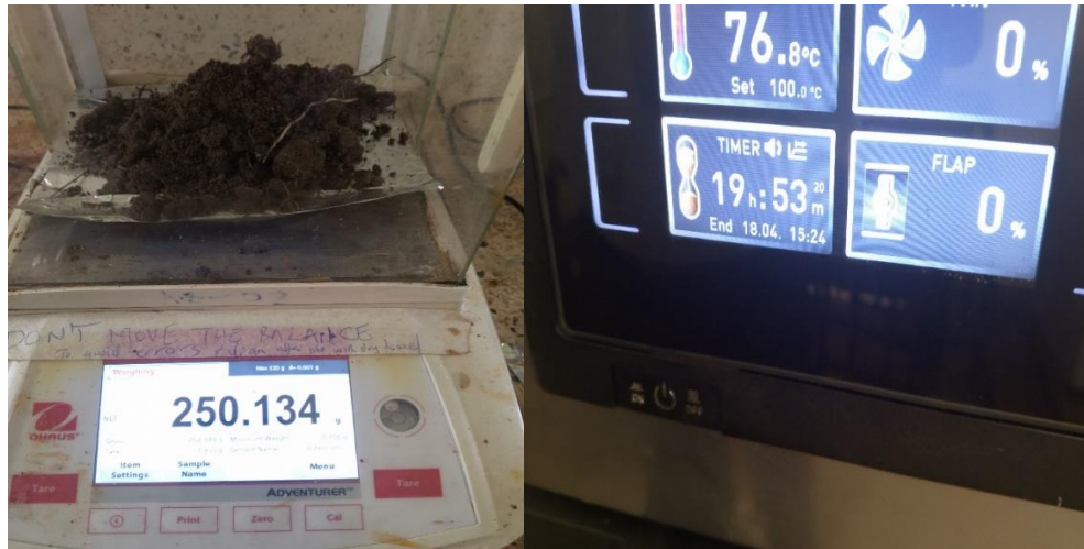
Figure 8; weighing and drying the soil sample.
