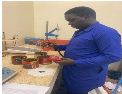
taking readings of moisture sensors
