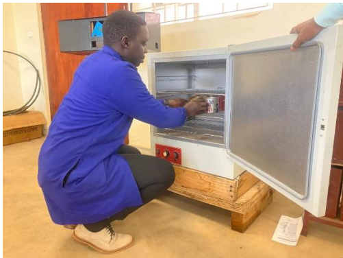
putting the soil samples in oven for drying
