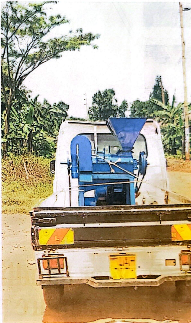
Costing Shs6.5m, the portable huller has the capacity to produce 500kg per hour, half the output of the traditional machines. PHOTO: OWEN WAGABAZA
