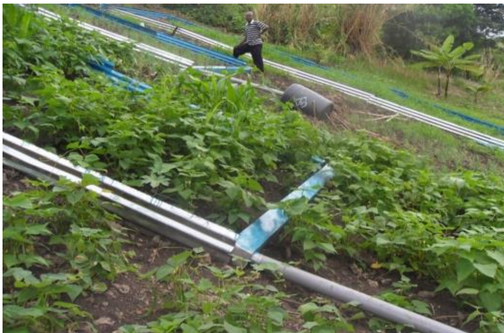
Plate 2. Erosion plot middle slope under Mixed cropping using Gerlach trough
