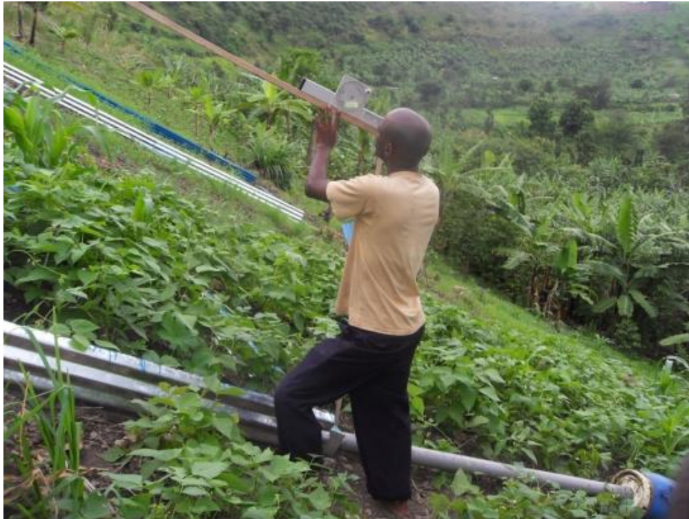
Plate 4. Measurement of slope angle by the researcher using an abney level
