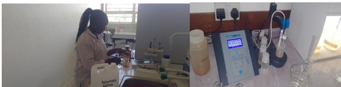
Figure 7.2: Raising and monitoring the pH using a pH meter and Sodium Hydroxide.
