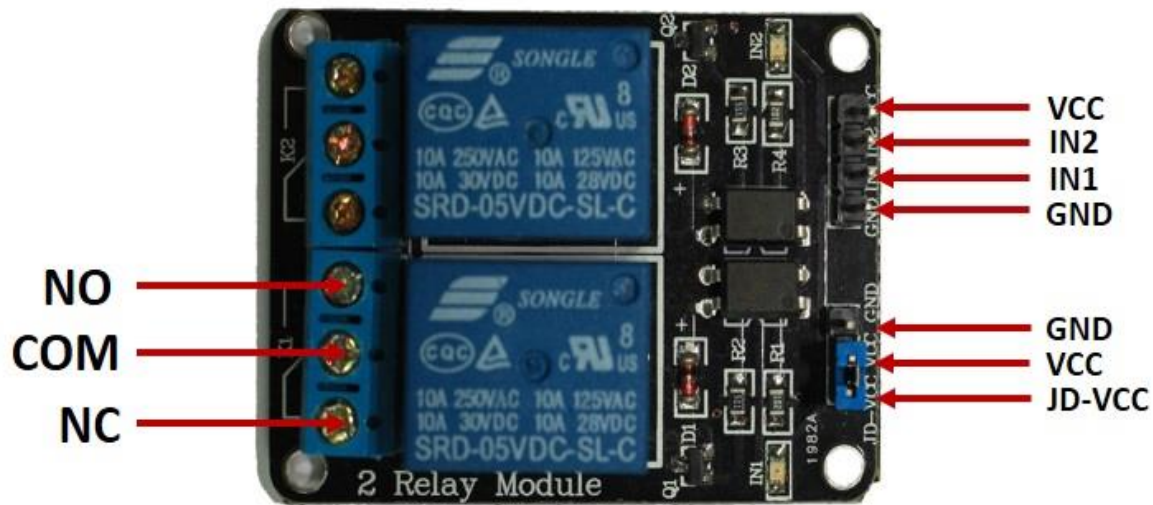
Figure 4 showing relay module
