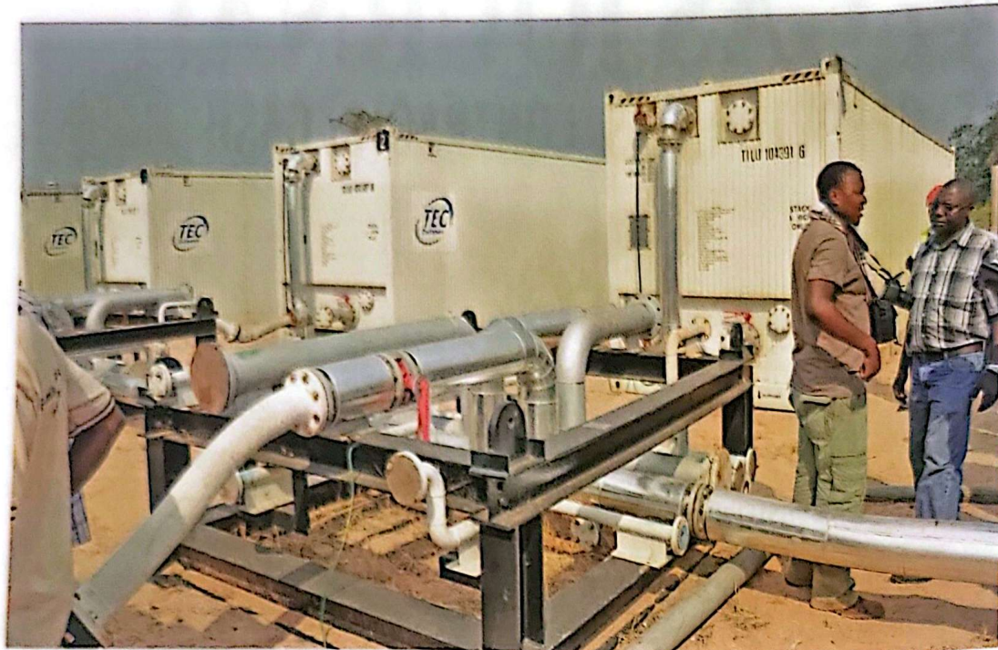
Bitumainers containing crude oil in the Albertine Graben. Previously crude oil produced during testing was flared
