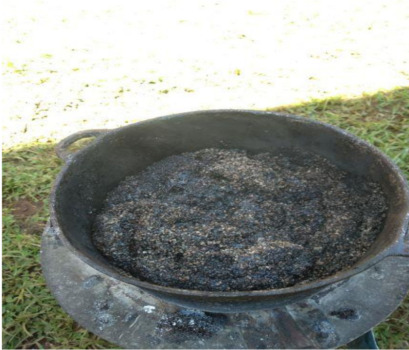
Figure 3.11: Mixture of Sand and Molten Plastic
