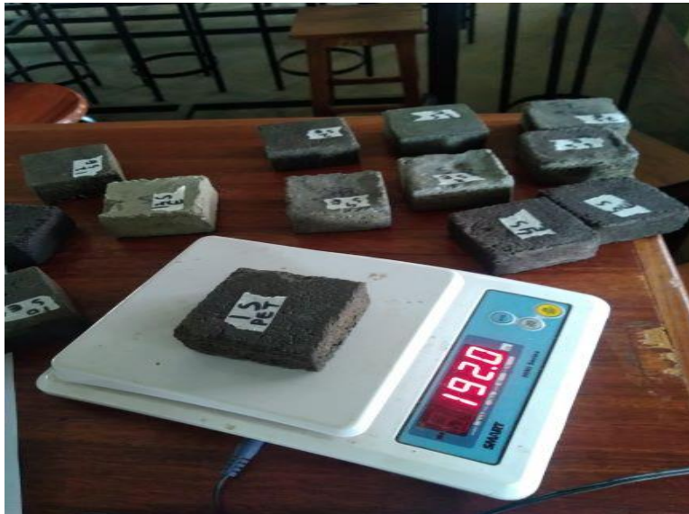
Figure 3.17: Measuring of mass of Paving Blocks using a Beam Balance
