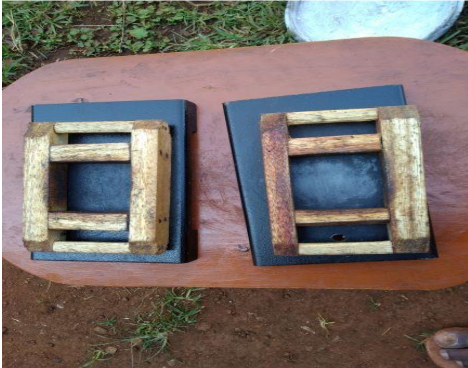
Figure 3.12: Molds Smeared with Used Engine Oil
