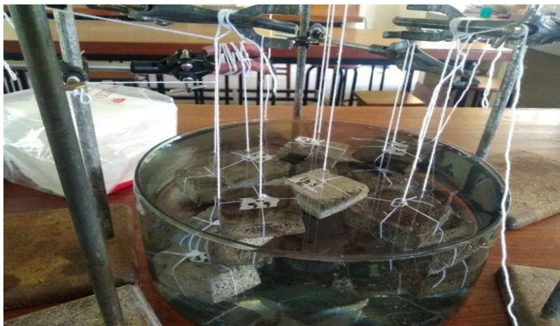
Figure 3.18: Paving Blocks Fully Immersed in Water
