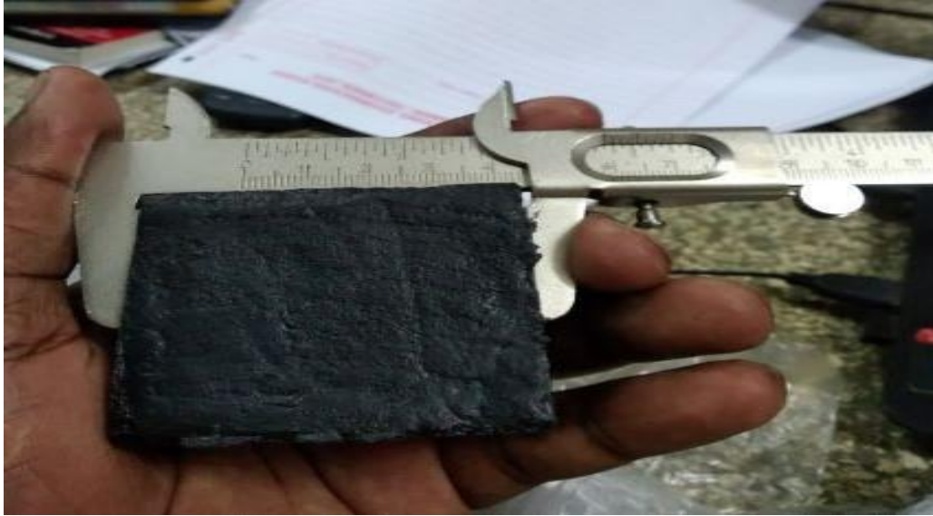
Figure 3.16: Measuring of sides of the Paving Block using Vernier calipers
