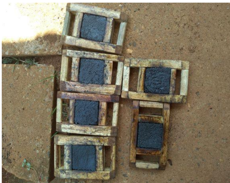
Figure 3.15: Pressed Mixture Left to Set and Cool
