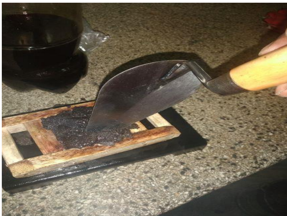
Figure 3.14: Pressing of Mixture in Mould
