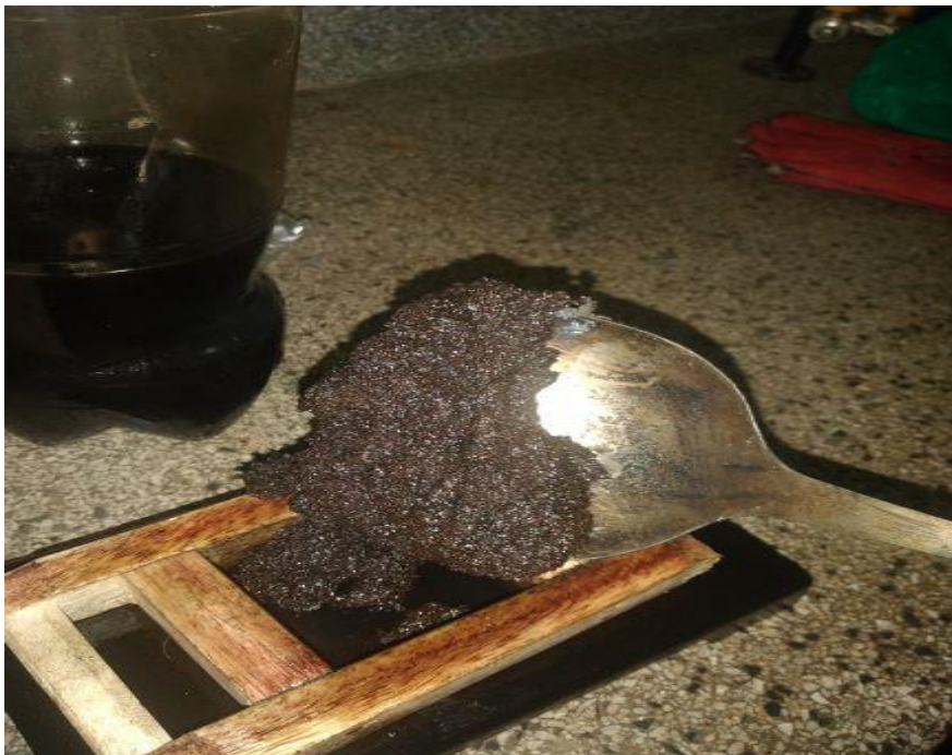
Figure 3.13: Placement of Mixture into Mould
