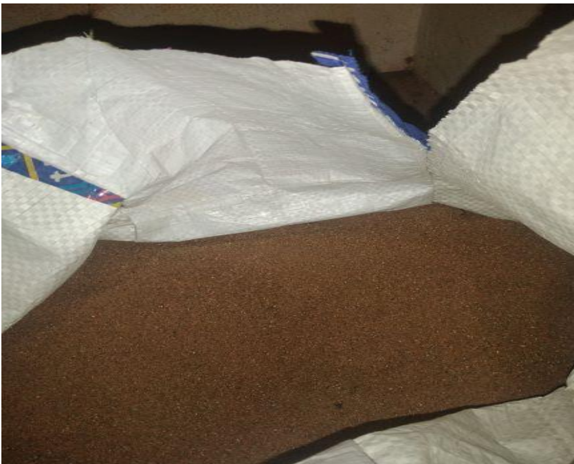
Figure 3.6: Sand Particles Passing Through a Sieve with 0.5 mm Pore Size
