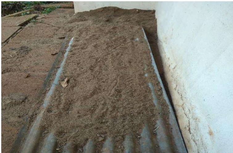
Figure 3.2: Sand Spread for Drying
