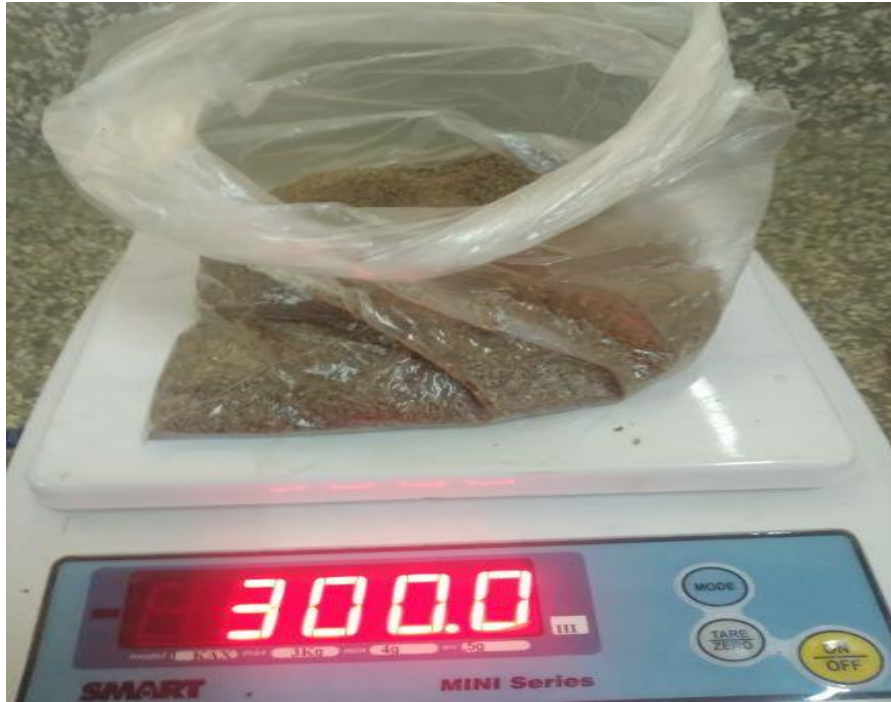
Figure 3.8: Measuring Sand Quantity
