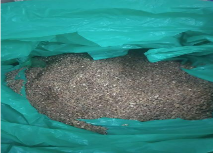
Figure 3.5: Sand Particles Passing Through a Sieve with 1.2 mm Pore Size
