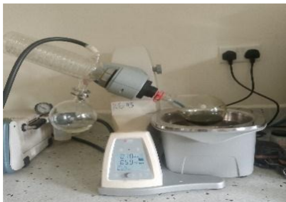
Figure 3; Rotary evaporator concentrating the plant extract by removing the solvent under reduced pressure.
