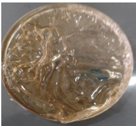
Figure 5 hydrogel of chitosan, gelatin and Musa acuminatum dissolved in water
