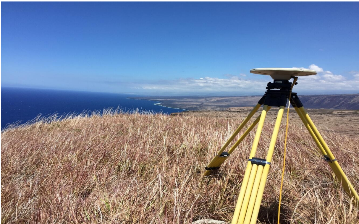
Figure 2.5: The GNSS receiver in an open place Adapted from https://www.usgs.gov/media/images/campaign-gps-antenna .
