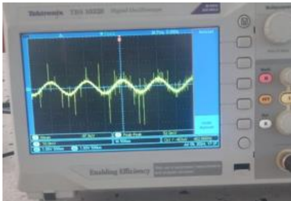
Figure 4.3 showing the CRO waveform when an egg carton was used.
