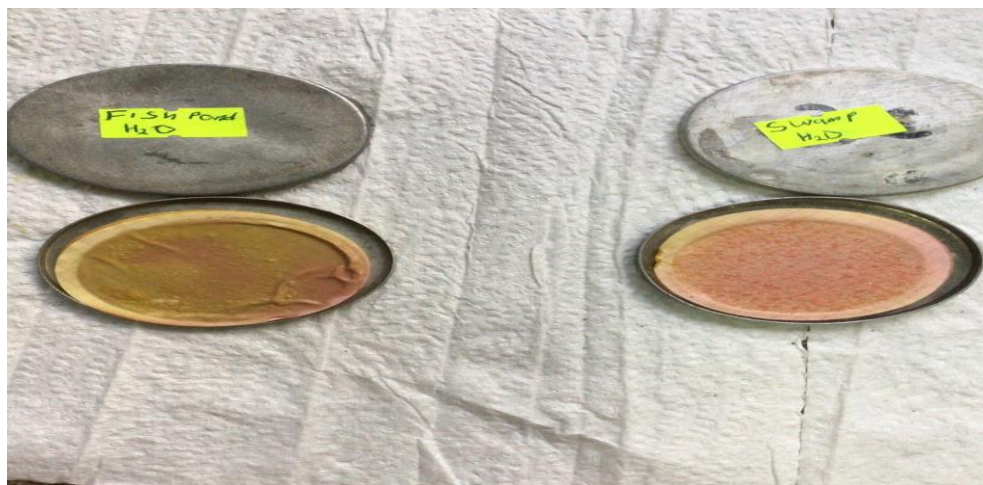
Figure 4.1 membrane filtration results showing TNTC total coliform growth for fishpond and swamp water samples
