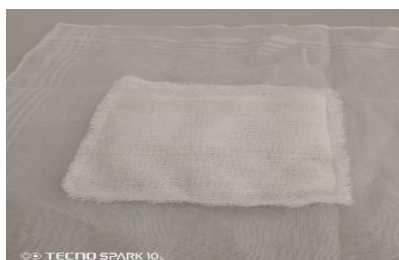
Figure 4.3stitched foam pad using plain gauze fabric (10cm widthx15cm length)
