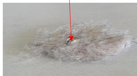
Figure 5.3: water drop above, indicating a more hydrophobic nature due to the presence of natural lipids and intact keratin structure, which limits water penetration.
