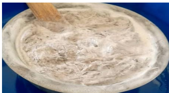
Figure 3.2: Fibres in sodium hydroxide solution
