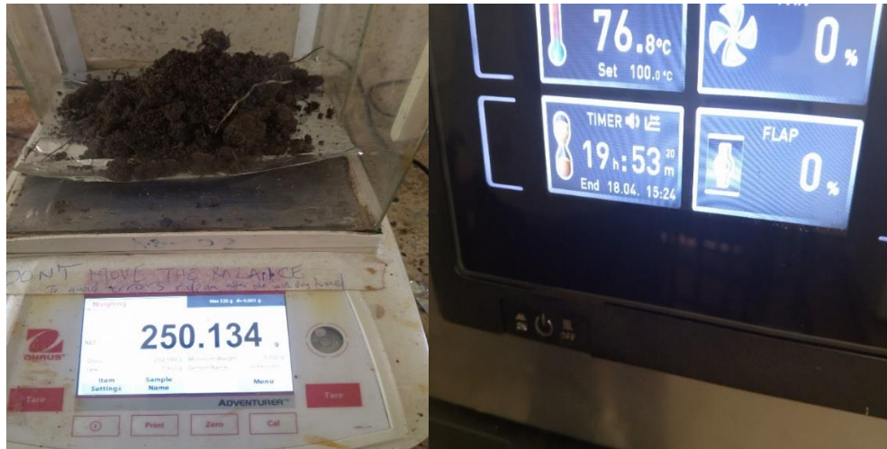
Figure 8; weighing and drying the soil sample.
