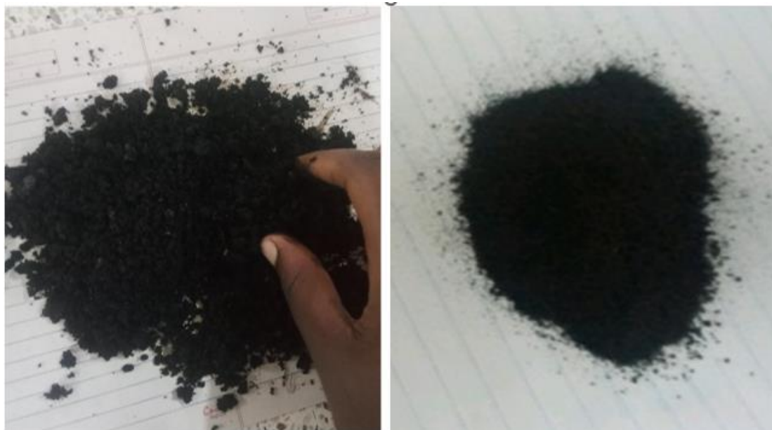
Figure 1: Activated carbon before and after drying
