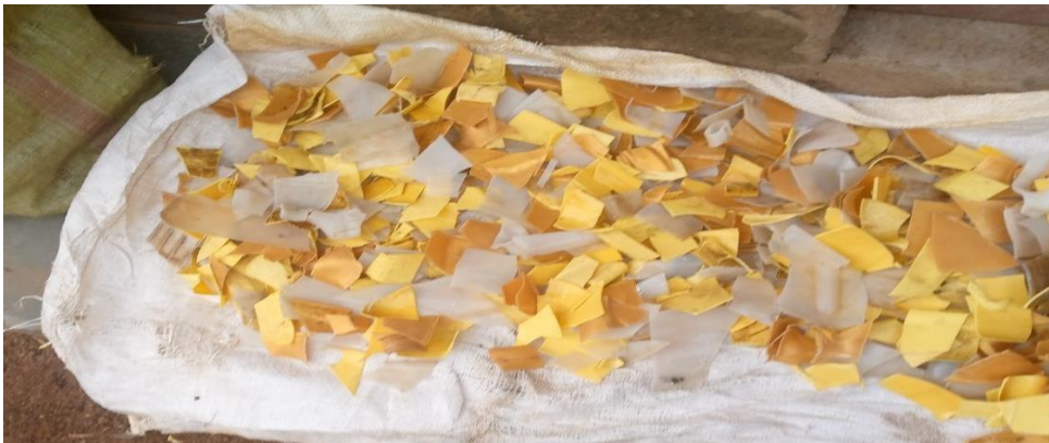
Figure 2. 4 Shows shredded high molecular weight plastic waste collected from Nagongera town
