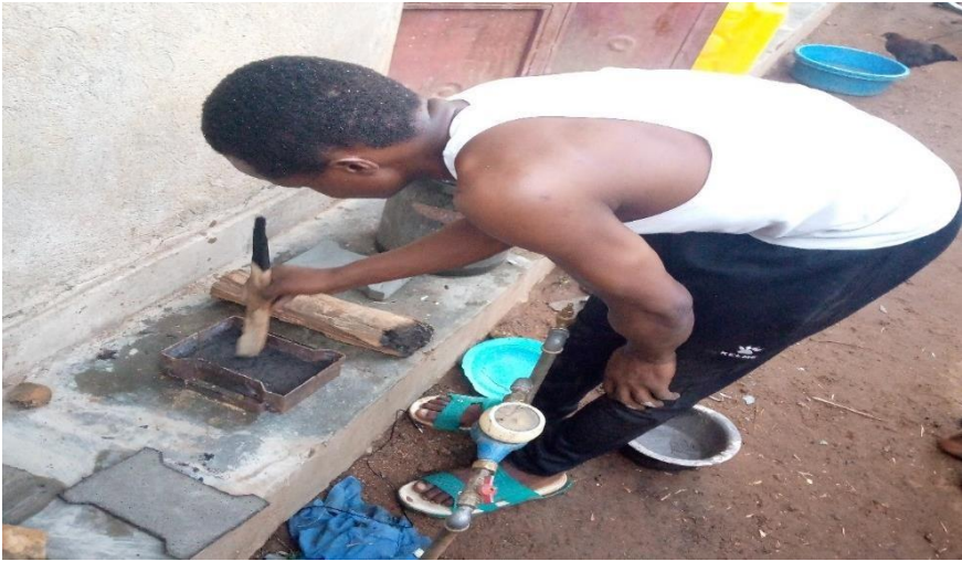
Figure 3.3.2 Molding of Plastic-Sand Mixture
