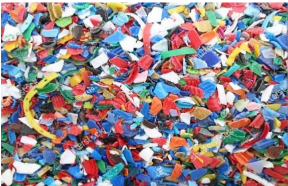
Figure 3.3.1. b Samples of Cleaned and Shredded Plastic Waste of HMD
