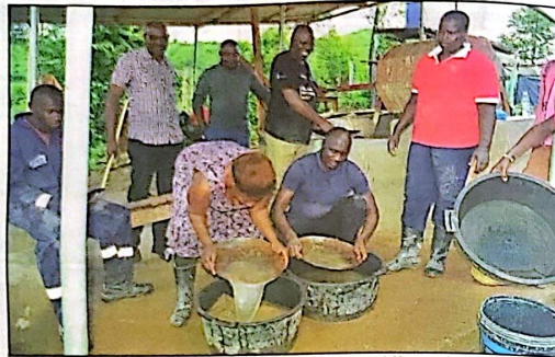
Artisanal miners using borax to purify gold concentrates at Kassanda mining site
